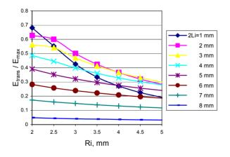
Figure 4: Iris radius  $\times E_{trans}/E_{max}$  for different iris lengths.
