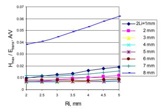
Figure 5: Iris radius  $\times$  H<sub>max</sub>/E<sub>trans</sub> for different iris lengths.
