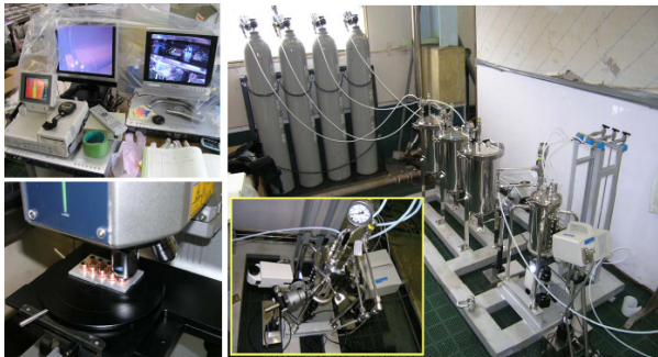
Figure 5: High-pressure (1~6 atm) chemical etching test stand for OFC-cathode tip plugs: the surface of the cathode tips was evaluated with a laser microscope.
