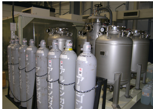
Figure 6: High-pressure chemical etching test facility for rf accelerating structures made of OFC.
