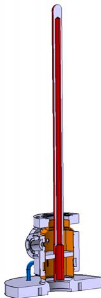
Figure 7: Updated design of the RF coupler.
