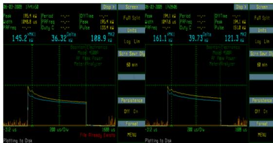
Figure 5: Before (left) and after bias current adjustment with pulse power meter.
