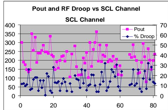
Figure 2: Klystron power and droop by SCL cavity.
