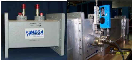
Figure 3 a, b: Waveguide Directional Coupler and 60 dB directivity modified unit.
