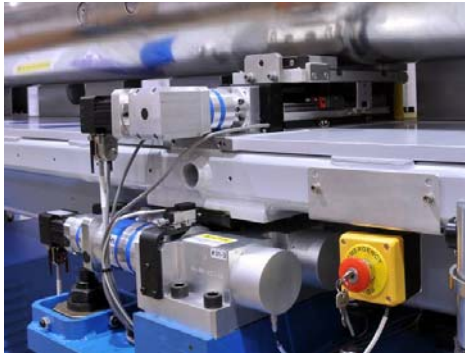
Figure 4: The undulator is mounted on a translation slide that is attached to the girder. The double CSM is shown below the girder, mounted on the intermediate plate.
