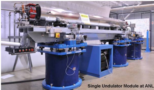
Figure 5: The single-undulator module at Argonne.
