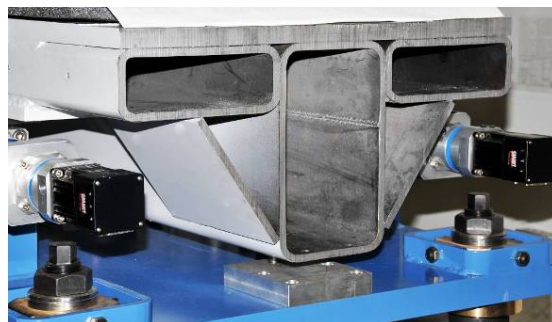
Figure 3: A cross section of the support girder mounted on the intermediate plate.
