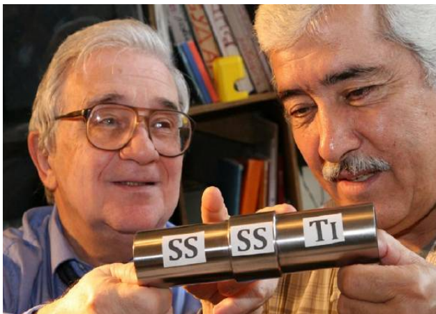
Figure 6: Explosion welding of bimetal tubes.
