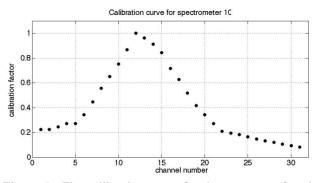
Figure 5: The calibration curve for the response of each segment of the segmented dump on spectrometer 10.
