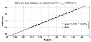
Figure 4: The horizontal dimension  $\pm 48$  mm for the segmented dump in spectrometer 10 corresponds to an energy spread acceptance of about 10%.
