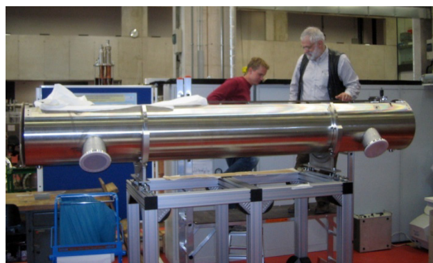
Figure 3: RFQ during assembly at IAP.
