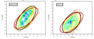
Figure 9: Contour plots show the horizontal and vertical phase-space distribution of a carbon beam from the RFQ linac (see text).
