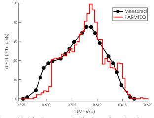
Figure 10: Kinetic energy distributions of a carbon beam from the RFQ linac. The filled dots and histogram show the results of the measurement and a PARMTEQ calculation, respectively.
