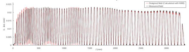
Figure 7: Electric field along the beam axis as functions of the beam coordinate, Z for the APF IH-DTL. The black and red curves show the measured and designed electric field, respectively. The designed field was calculated with MWS.
