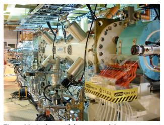
Figure 14: A picture of the compact injector system, as installed in the injector room of the HIMAC.
