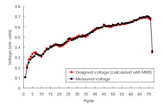
Figure 8: Gap voltages along the beam axis as functions of the gap number for the APF IH-DTL. The black and red dots show the measured and designed voltage, respectively.
