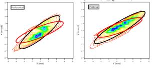
Figure 11: Contour plots show the horizontal and vertical phase-space distribution of a carbon beam from the APF IH-DTL (see text).
