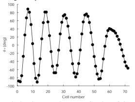
Figure 2: Synchronous phase as a function of the cell number.
