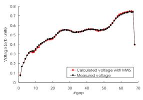
Figure 5: Gap voltages along the beam axis as functions of the gap number for the model cavity. The black and red dots show the measured and calculated gap-voltages, respectively.
