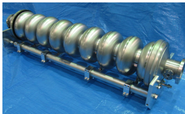
Figure 2: 1.3GHz superconducting 9-cell cavity with new techniques. (MHI-#A).
