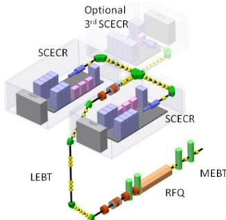
Figure 2: Layout of the double-folded driver linac front end.
