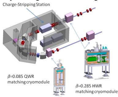
Figure 5: The layout of Folding Segment 1 and required matching cryommodules.
