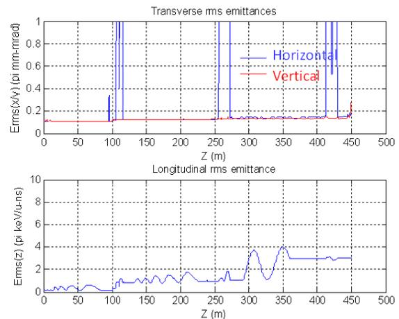
Figure 7: Uranium beam transverse (top) and longitudinal (bottom) emittances along the SC driver linac.
