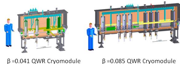
Figure 3: QWR cryomodules used in double-folded SC Linac Segment 1.
