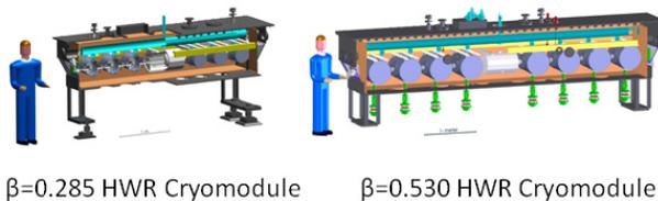
Figure 4: Two types of HWR cryomodules used in double-folded SC Linac Segment 2.
