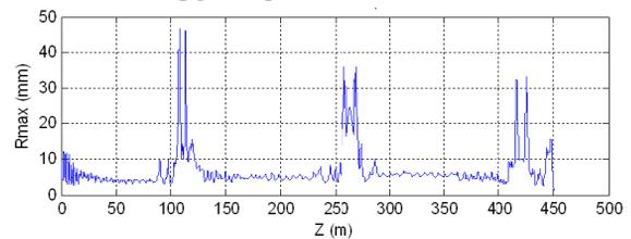
Figure 6: Uranium beam envelope along the SC driver linac.
