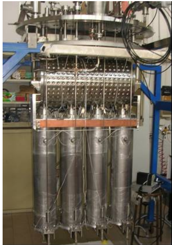
Figure 1: The low- \beta cavities in the prototype cryostat.
