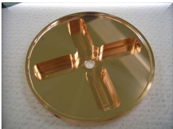
Figure 2: Photo of a damped cell used for the TD18 structures.
