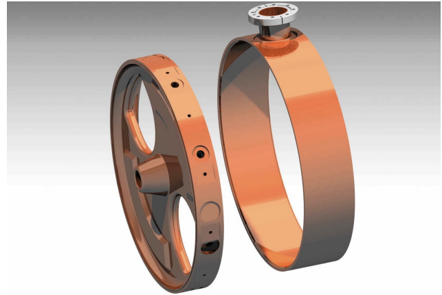
Figure 1: Discs and rings before welding.
