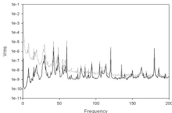
Figure 3: Cavity 1 phase noise.
