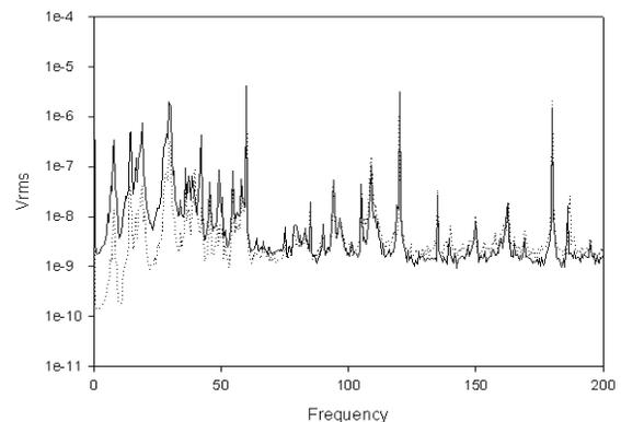
Figure 4: Cavity 4 phase noise.
