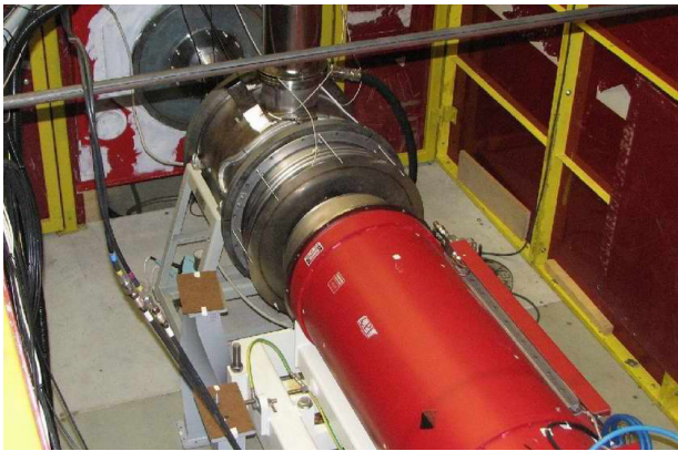
Figure 7: CPI 1.3 GHz, 10 MW MBK “VKL 8301B”.
