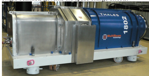
Figure 6: Thales 1.3 GHz, 10 MW MBK “TH1802”.
