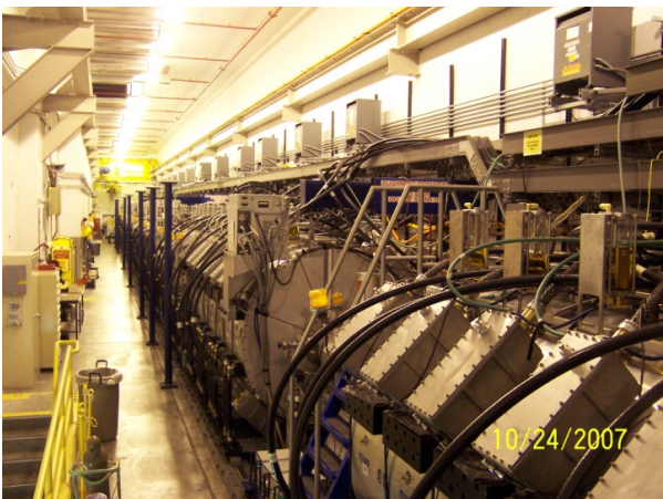
Figure 3: An end-view of the DARHT Axis II accelerator hall showing the linear string of accelerating cells.
