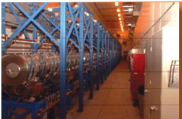
Figure 2: An end-view of the DARHT Axis I accelerator hall showing the linear string of accelerating cells.
