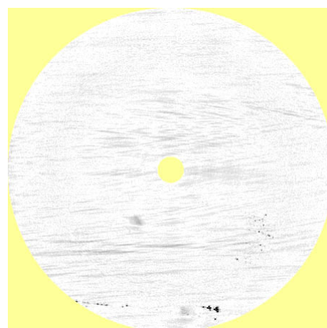
Figure 5: Scan image of a sheet with iron inclusions, old device.
