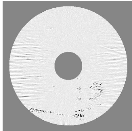
Figure 4: Scan image of a sheet with iron inclusions, new device.
