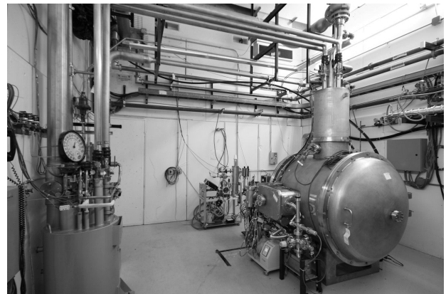
Figure 1. Photo of the Cavity Test Facility Cryostat
