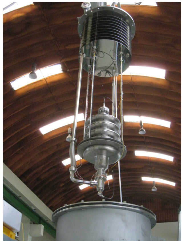
Figure 6: Cavity installed in the insert of the cryostat.
