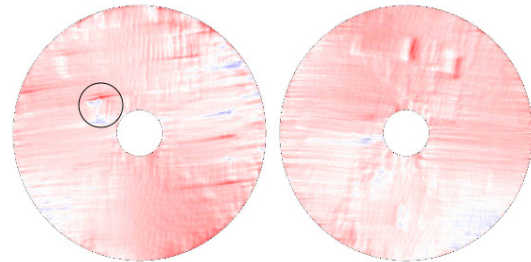
Figure 5: Typical results of the eddy-current inspection. Both side of a niobium disk before the cup forming for SC cavity were measured. Surface at a circle is comparatively rough.
