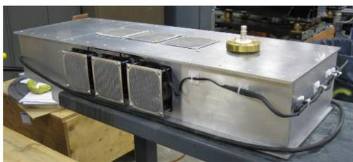
Figure 4: Isolation transformer.
