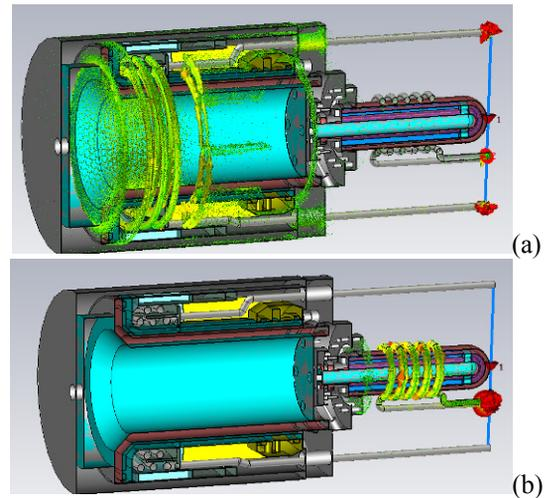
Figure 3: RF modeling of external antenna ion source with separate 13.56 MHz antenna: (a) Surface current at 2 MHz, (b) Surface current at 13.56 MHz.
