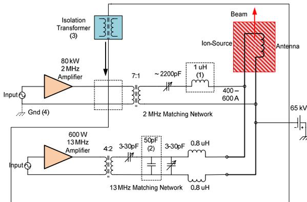
Figure 2: SNS ion source RF system. An isolation transformer (3) is inserted between the 2 MHz amplifier and the impedance matching transformer.
