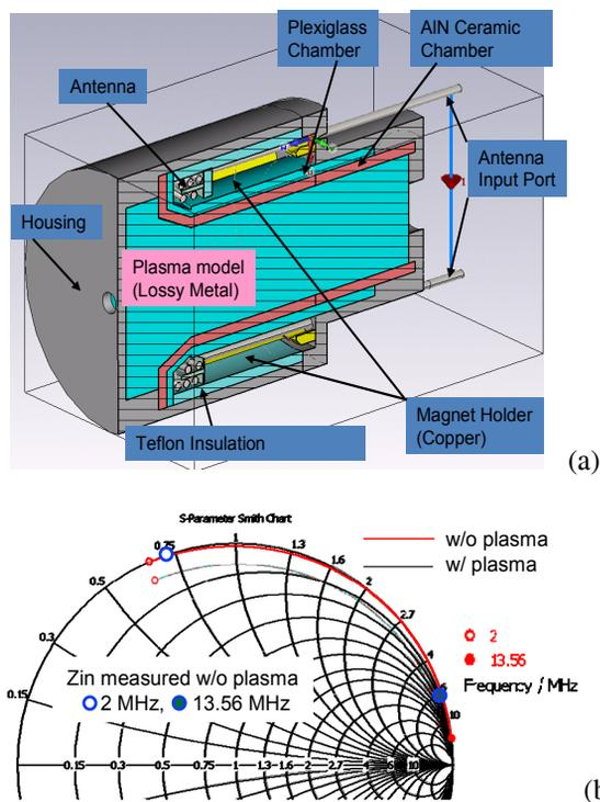
Figure 1: (a) External antenna ion source, (b) computed input impedance of the external antenna.
