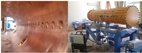
Figure 6: Prototype of the first unit DTL tank.
