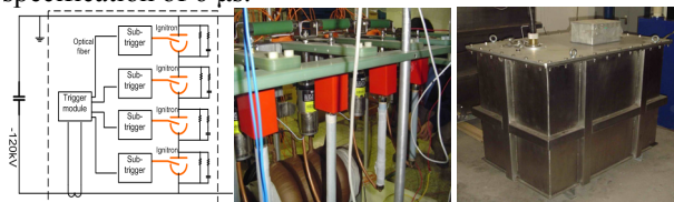
Figure 16: Block diagram (left), internal (middle) and external structure (right) of CSNS crowbar.
