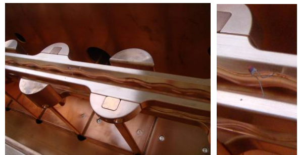
Figure 3: Estimation of shunt impedance with a perturbation capacitor.
