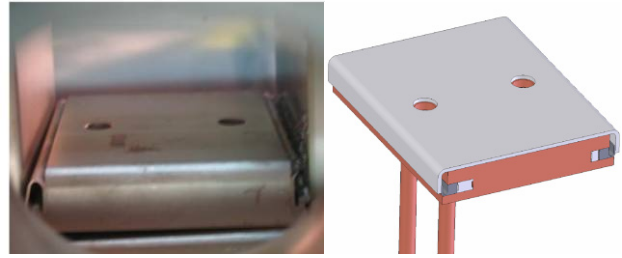
Figure 13: The burned 70 \times 2\ \mu\text{m} silver plated Inconel spring contact due to poor heat conductivity of the former tuning plate and the new design with a massive brazed 1500\ \mu\text{m} silver plate on top of the tuning plate.
