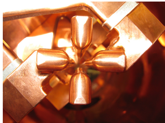
Figure 2: A picture of the four RFQ electrodes at the radial matcher.
