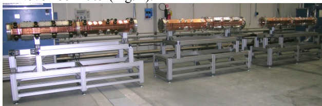
Figure 1: The complete TRASCO RFQ structure assembled at LNL.
