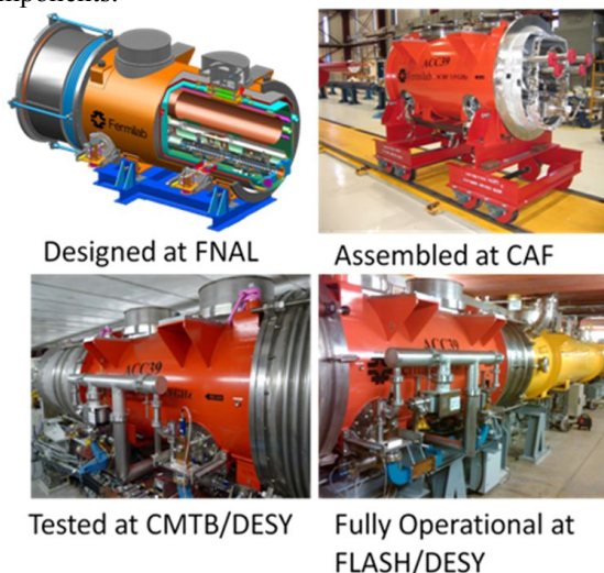
Figure 2: 3.9GHz cryomodule from design to successful operation at FLASH.
