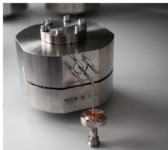
Figure 4: 1.3 GHz cavity dark current monitor with one coupling antenna in front.
