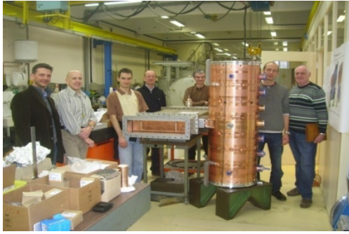
Figure 12: The PIMS cavity vertically assembled at the CERN Workshop.
