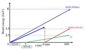
Figure 5: Beam energy variation along linac in the ordinary operation scheme.
