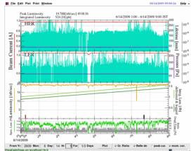
Figure 15: Stored beam current of HER (top), LER (middle), and luminosity (bottom) of KEKB in the simultaneous top-up operation (24 hours).
