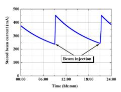
Figure 3: Stored beam current of PF in the original injection operation (24 hours).
