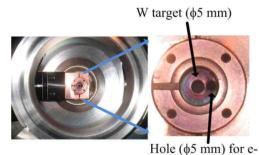
Figure 12: Photograph of the new positron production target with a hole.
