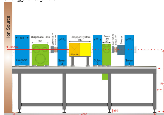
Figure 4: Scheme of the LEBT section with four solenoids and the chopper device.
