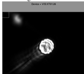
Figure 2: Virtual cathode image (4x6 mm): the main spot is the non-attenuated UV and the upper left spot is the green laser attenuated with filters.
