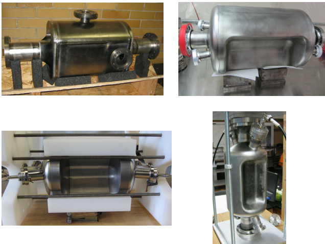
Figure 16: Prototype of the 400 MHz 4-rod cavity (top left), 400 MHz (top right), 400 MHz (bottom left) and 750 MHz (bottom right) rf-dipole cavities.
