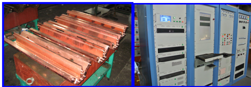
Figure 9: RFQ vanes under fabrication (right) and tetrode power source (left).
