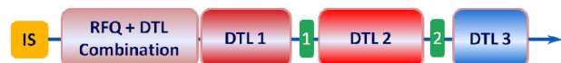
Figure 1: Structural scheme of the NICA injector of light and polarized ions. (IS – ion sources)/
