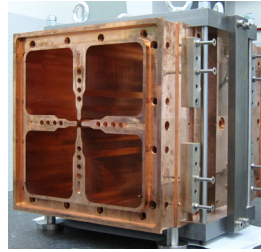
Figure 7: Module 16 dry assembled before the machining of the common planes
