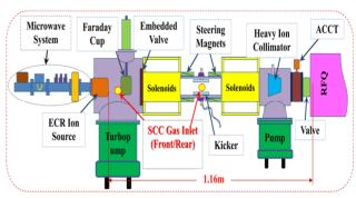
Figure 3: Schematic view of the helium injector.
