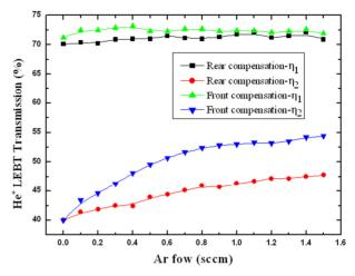
Figure 2: LEBT transmission of  $30 \text{keV}/65 \text{mA He}^+$  beam with front compensation and rear compensation.
