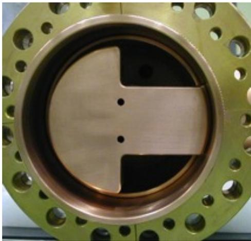
Figure 2: Rf coupling loop of DTL
