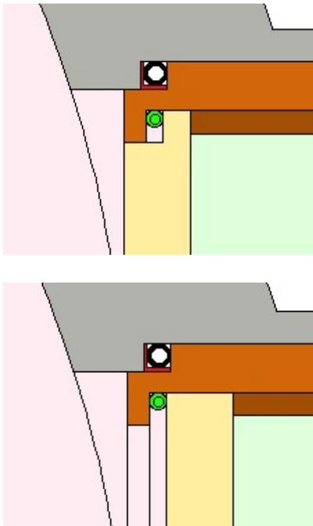
Figure 7: Cross sectional view of the cerarmic window Yellow:window, Brown:outside cylinder of the waveguide Green:vacuum seal, Red:rf contact, Gray:cavity wall
