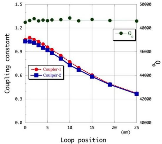
Figure 8: Measured coupling constant for DTL1 [2].
