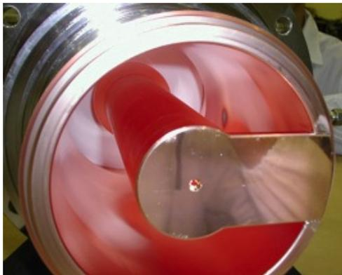
Figure 3: Rf coupling loop of SCTL
