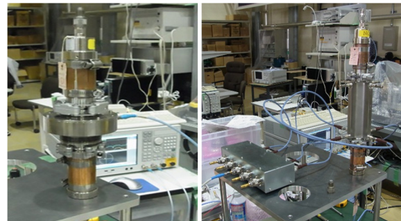
Figure 3: Overview of the test bench. An FCT is set on left side and a BPM is set on right side.
