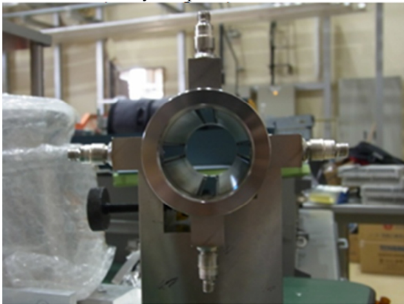
Figure 2: Beam Position Monitor (BPM).
