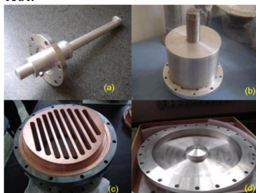
Figure 6: Aluminium cold models: post coupler (a), slug tuner (b), vacuum grill (c) and end wall (d).
