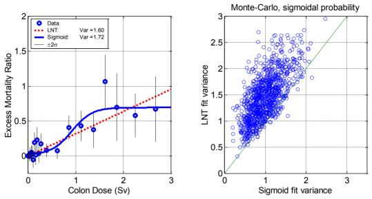
Figure 1: The cancer mortality of the survivors can be described by an s-shaped dependence on radiation exposure with a threshold of about 0.3 Sievert (Sv) and saturation level at about 1.5 Sv; such description is not worse than the linear one (left). Moreover, Monte-Carlo simulation of possible outcomes demonstrates that, given the weak statistical power, the follow-up cannot provide support for LNTH (right). Source: Socol and Dobrzyński [3].
