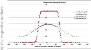
Figure 10: Transmission through the DTL tank1 vs. DTL phase for bunchers off and bunchers on.
