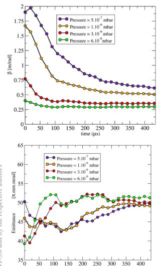
Figure 5: Twiss beta parameter (top) and un-normalised emittance (bottom) along the beam pulse for different pressure in the LEBT.
