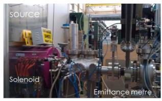
Figure 2: Set-up for emittance measurements at 45 keV.
