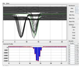
Figure 8: Beam transverse profile on the wire scanner before the in-line dump. Top: A profile (solid black line) is taken every  $6~\mu s$ . Bottom: Profile of a slice of the main beam. Horizontal scale in mm, vertical a.u..
