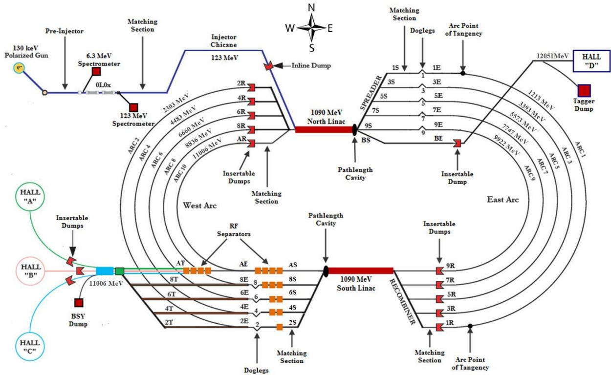
Figure 2: Schematic representation of the CEBAF accelerator with nominal energies shown for a 12 GeV configuration.
