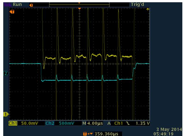
Figure 4: Oscilloscope trace showing 6 beams for the first time in the NL as measured by a linac  $M_{56}$  cavity.
