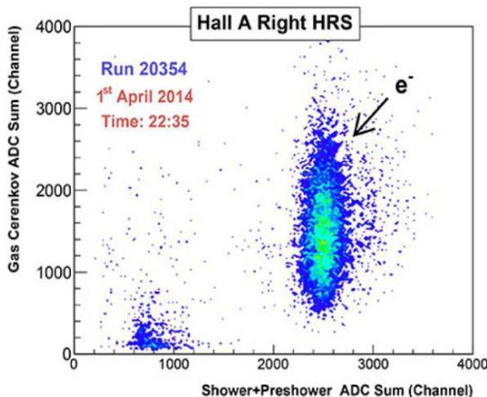
Figure 3: First CW electrons detected in the Hall A High Resolution Spectrometer.
