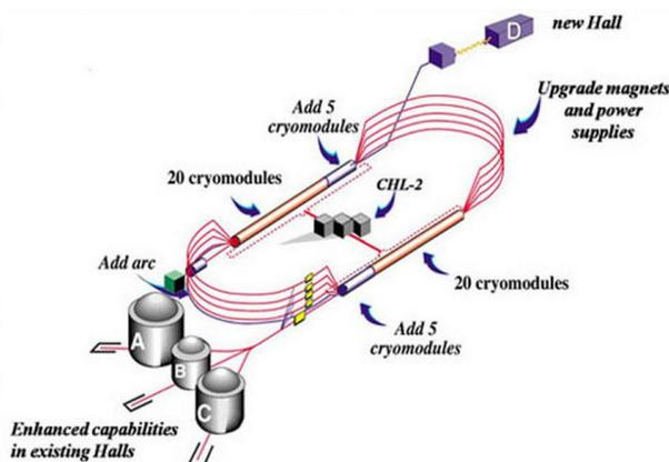
Figure 1: Schematic representation of the CEBAF accelerator showing the original configuration along with the major components of the upgrade.
