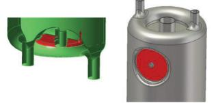
a) Electric region b) Magnetic region Figure 4: Slow tuner mechanisms (red – deformation area)
