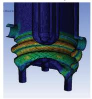
Figure 5: Von Mises stresses distribution for bellows tuner
