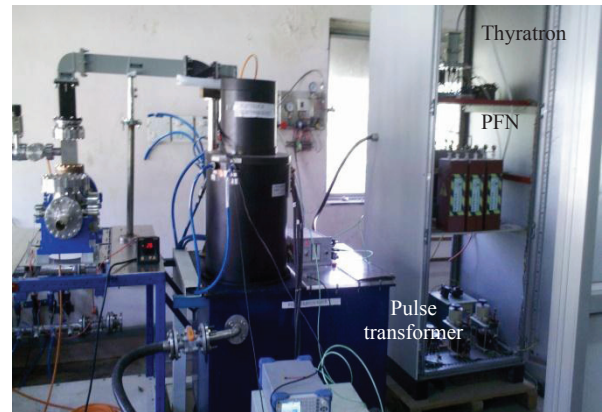
Figure 6: Modulator with single-beam klystron on test
