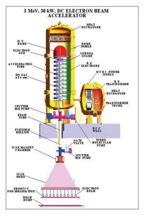
Figure 1: Schematic of 3 MeV DC Accelerator
