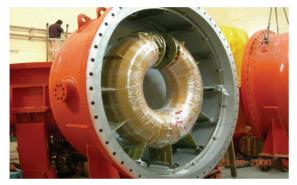
Figure 3: Transformer installed inside pressure vessel
