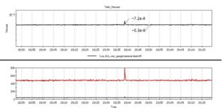
Figure 6: Rise in detector (Sc-2) counts during pressure spike due to ion pump in Tank 1.
