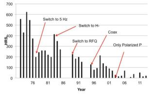
Figure 1: Total linac down time in hours since 1972 for HEP and RHIC operations.
