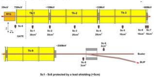
Figure 4: Detectors placement along the linac. Detectors have volume of 30, 20 10 and 2 cm<sup>3</sup> for tank 1,2 3 and BLIP bending magnet 1 respectively.
