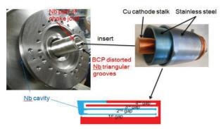
Figure 2: Quarter-wavelength cathode stalk insertion.
