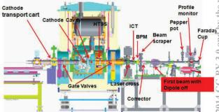
Figure 6: First beam commissioning configuration.
