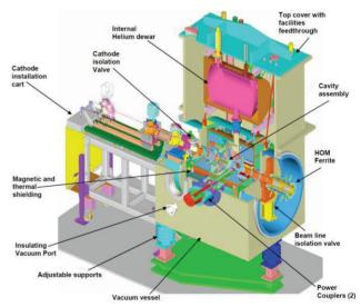
Figure 1: SRF gun cryomodule.
