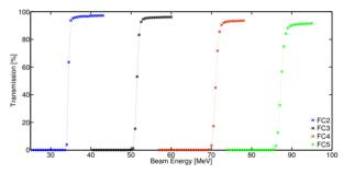
Figure 4: Transmission in the FC as function of the beam energy for the last four FC.
