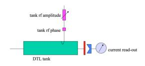
Figure 1: Schematic of the energy degrader method from phase scan measurement in the DTL, the energy degrader is represented in red and the charge collector in blue.
