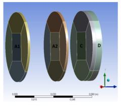
Figure 3: Example of FC geometry in FE code, A1 is the first foil, A2 the second and C the collector.
